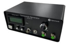
WTEC-01-25 is a Fabry-Perot Electro-Optic (FP-EO) optical frequency comb generator with high frequency stability and low phase noise. The components are all passive so that the comb stability and comb interval are equal to input laser and modulation frequency (RF) respectively. Hermetic sealed waveguide FP-EO modulator/OFCG-2.5-25AS is built-in for comb/pulse generator to realize high performances and high reliability. Temperature control unit is built-in WTEC-01-25.
