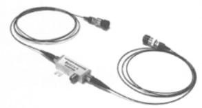
OFCG-2.5-25AS is a waveguide Fabry-Perot Electro-Optic (FP-EO) modulator which is optimized to output comb lines at a 25GHz spacing. A higher modulation efficiency and a higher optical finesse results in a typical comb span that can reach 10THz. The comb stability is related to the optical and RF input stability. This device can generate ultra precise optical comb/pulses with low phase noise and low timing jitter.
